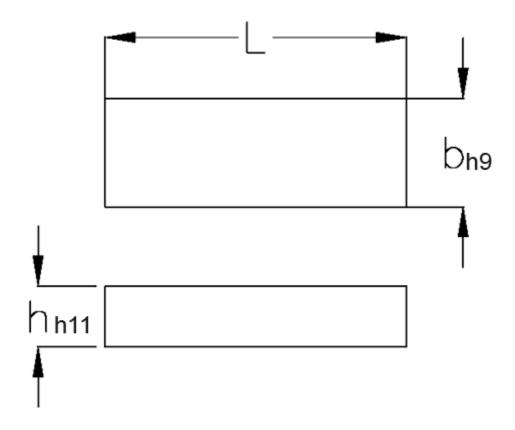
b = 8 h = 5 L = 40 Tolerance b = 0.036 Tolerance h = 0.075
